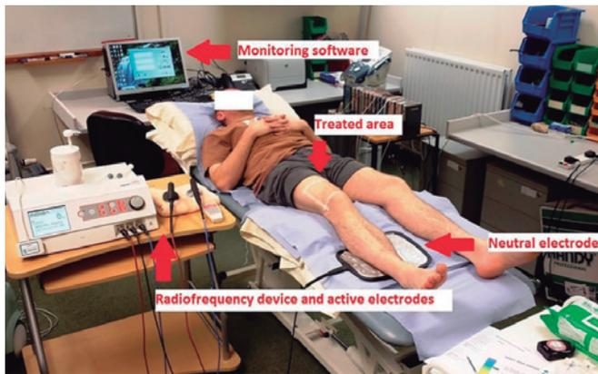
Figure 1. The experimental setting with the 448 kHz capacitive resistive monopolar radiofrequency (CRMRF) device (INDIBA®), electrodes and the computer based monitoring software.
